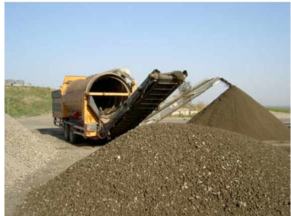
Figure 2. Screening shapes the SLAGsand to fit the other components.
