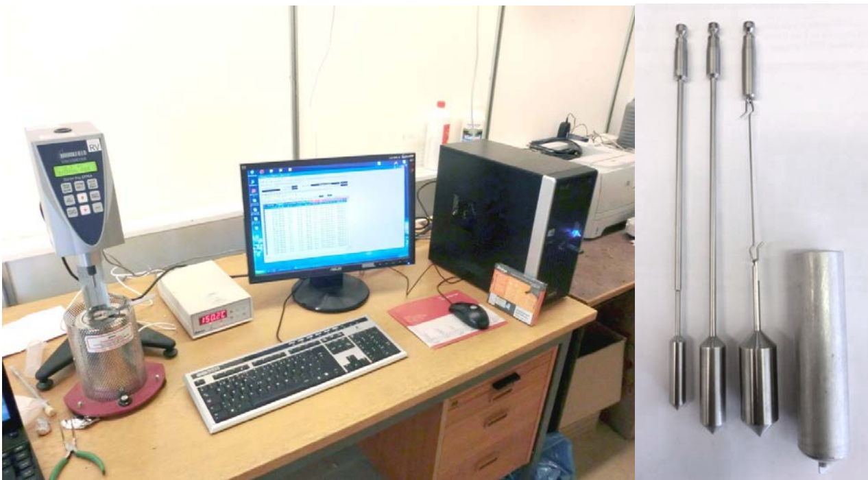
Figure 1: The RVB-equipment: viscometer, electrical heating device and computerized control of running the measurements and recordings. To the right rotating spindles, from left #29, #27, #21 and a cylindrical test container.
